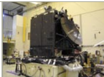
Rosetta spacecraft undergoing vibration testing.
