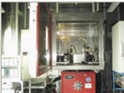
Fuel injection system undergoing combined climatic/vibration qualification testing in operating conditions.
