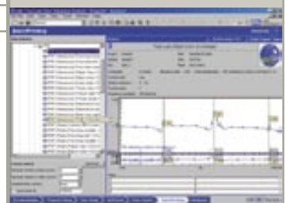
Fully automatic batch plotting at the end of test run, including automatic peak cursors.
