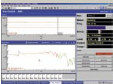
Test progress monitoring with drag and drop overlay of saved and life data.
